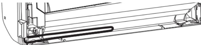
Run the connecting cable in the space on the back of the unit as shown in the above figure.
