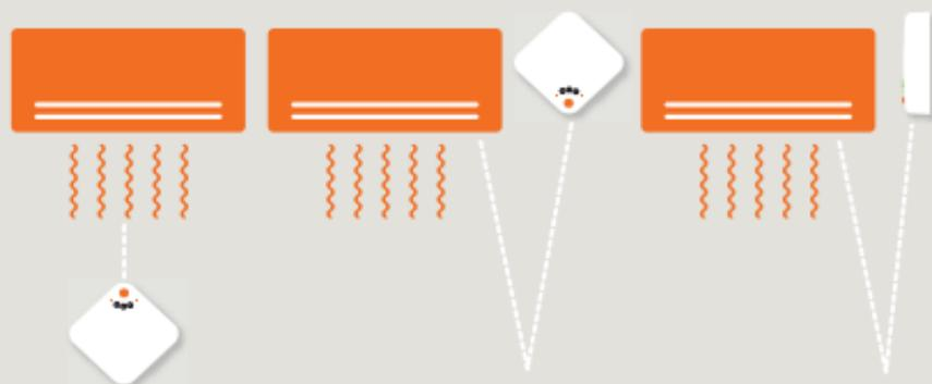
(Other mounting configurations are possible too as long as IR transmission from the controller to the heat pump works.)
